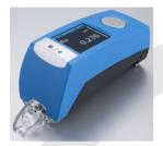
The right surface roughness on a gravure cylinder is not only decisive for a long lifetime of the cylinder but also for a smooth printing performance. Thanks to the Rz-Star measurement device you can now check your roughness in a matter of seconds. Additionally you can print out the measured values with the optional Bluetooth printer as evidence of your high quality standards.
